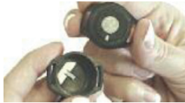
Removing the old batteries
