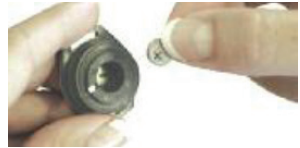
Inserting the new batteries
